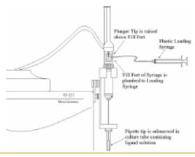
Picture adopted from 6 VP-ITC MicroCalorimeter User's Manual, p. 43
