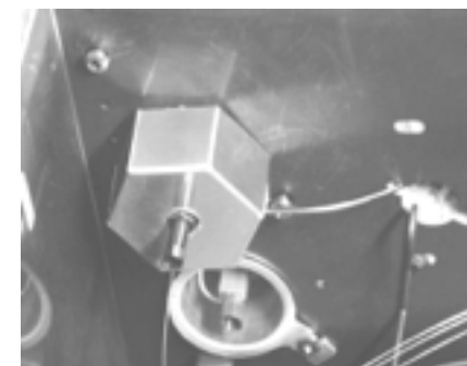
Install the adapter at the outlet of the GC injection port
