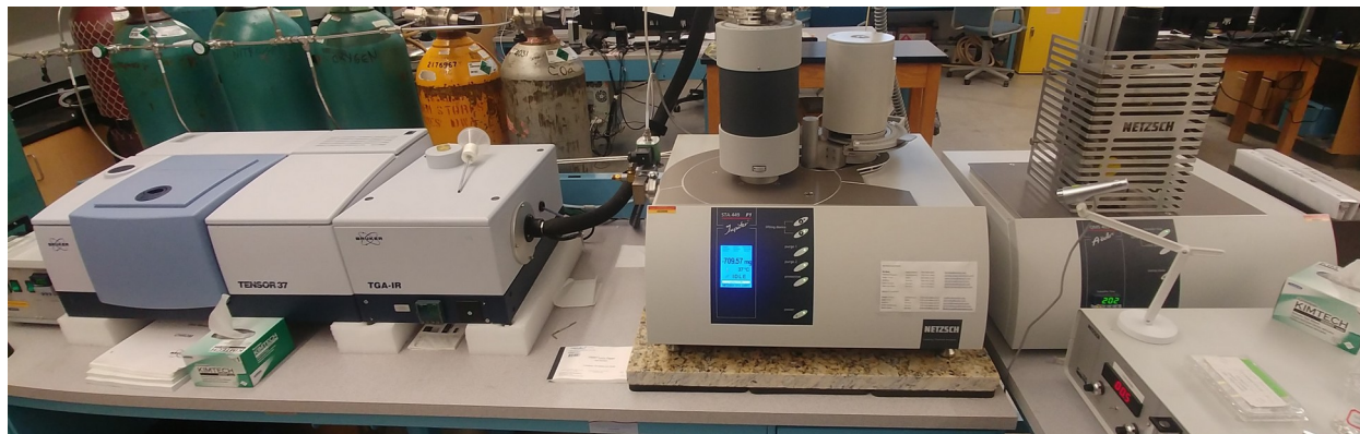
Fig.1 Netzsch STA449F1 TGA/DSC System with IR and MS
