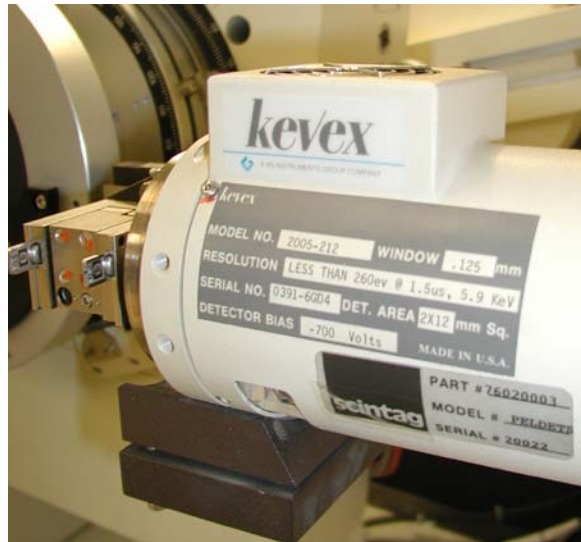
Fig. 4. The slits positions on a X-ray housing and detector.
