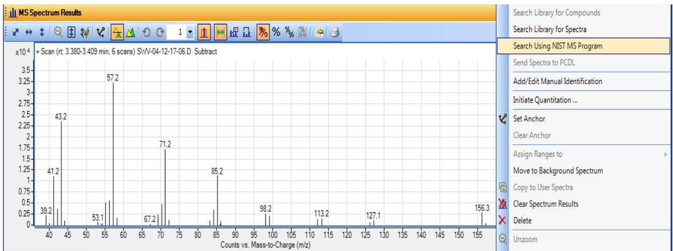
This will call the same NIST search algorithm used by the ChemStation processing program. You may also select "Search Library for Spectra" which uses the Agilent probability-based-matching (PBM) algorithm.
