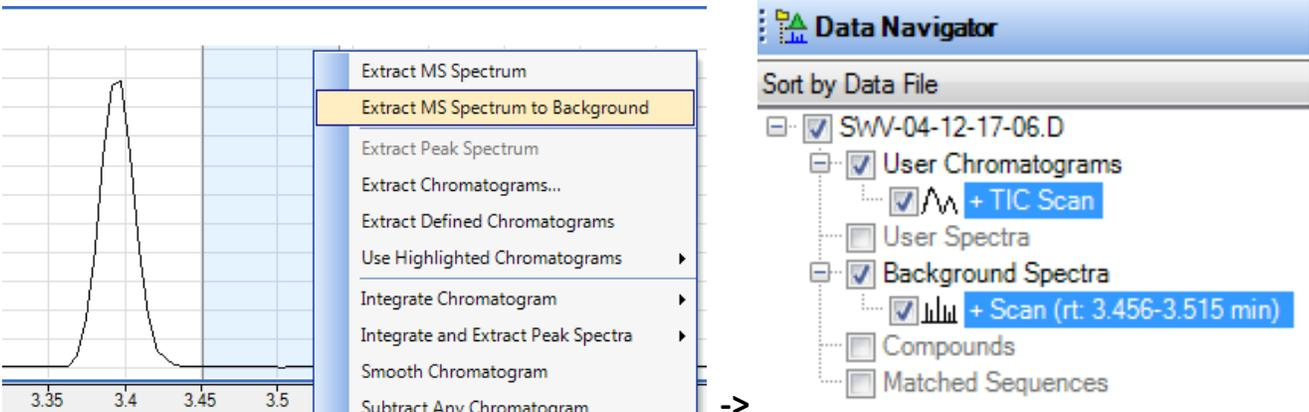
The screenshot shows a chromatogram with a peak at approximately 3.45 minutes. A context menu is open over the peak, with the option "Extract MS Spectrum to Background" highlighted. To the right, the "Data Navigator" window shows a tree view of data files. Under "SwW-04-12-17-06.D", the "Background Spectra" folder is expanded, and a scan labeled "+ Scan (rt: 3.456-3.515 min)" is highlighted in blue.
