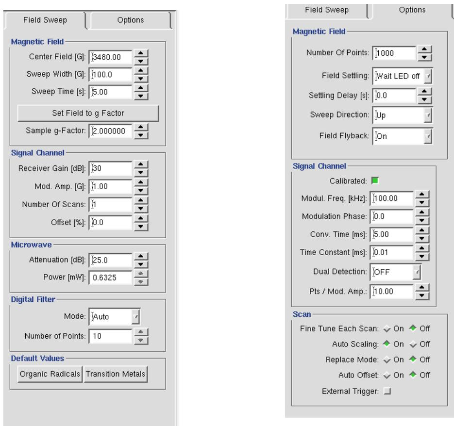
Figure 2-32 Initial default parameters.
