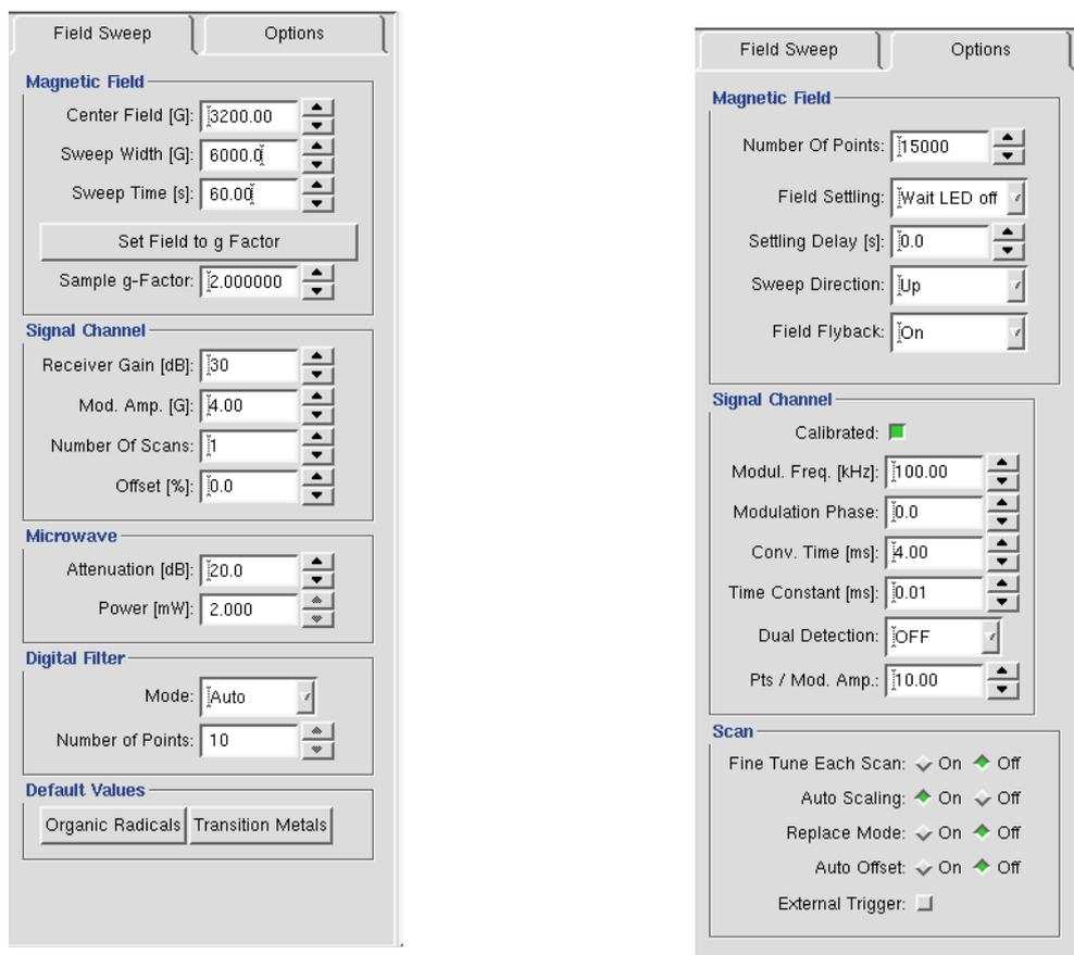
Figure 2-34 Default spectrometer parameters for transition metal samples.
